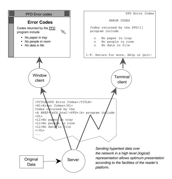
Fig. 3: A schmatic illustration of the encoding of hypertext data. The link is represented in the winodw by underlining, on the terminal by a reference number.
