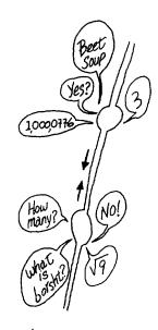
A given, pair of nodes may exchange Several independent messages for simultaneous user with different interests
